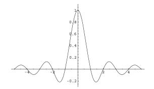
As  $\hat{f}(u) = 0$  at  $u = \pm 1, \pm 2, ...$  these frequencies are erased in the filtered image. Considering the envelope of the Fourier transformation of f, one directly observes that high frequency bands are damped the most.
