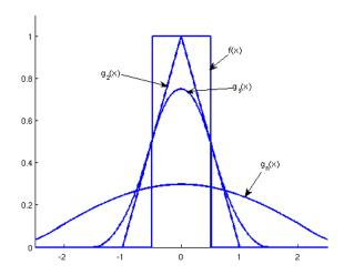
Convolution of two box filters results in a tent filter (piecewise linear). Subsequent convolutions then yield piecewise quadratic, piecewise cubic, etc. filters, which in the limit converge to a Gaussian filter.
