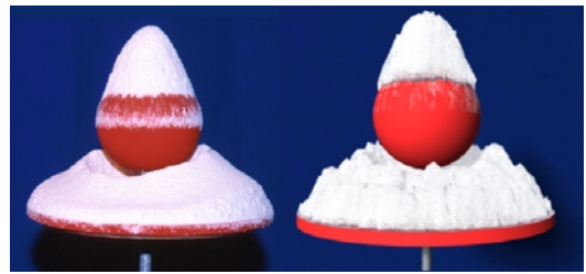
Figure 15: A real flour-covered scene (a) and a computer generated scene (b) compared to show that our stability algorithms are at least plausible. Our experimental setup was fairly ad-hoc: despite our best efforts, flour was distributed unevenly around the base of the real sphere.
