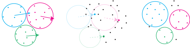
Figure 4: The cluster velocities at time t_k (left) are used to predict the cluster positions at t_{k+1} (center). Assigning 3D points to the closest predicted centers (right) yields a partial clustering at t_{k+1} . The non-clustered points (black) are then clustered in an independent step.
