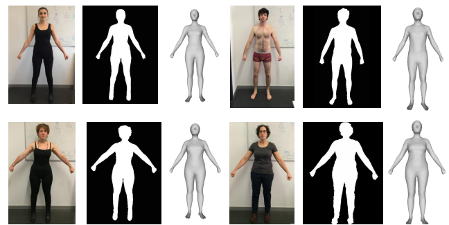
Figure 5: Mesh reconstruction for 4 real subjects in mildly varying poses. (left) Input image (middle) Extracted Silhouette (right) Reconstruction of the estimated shape.
