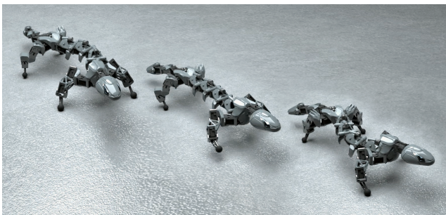
Figure 8: Salamander: our framework automatically generates swaying tail and spine motion, leading to a natural-looking gait.
