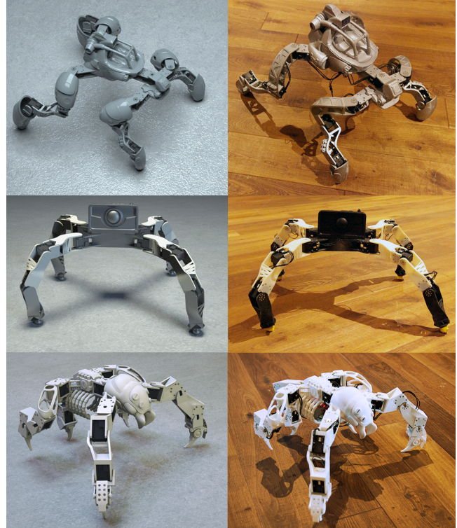
Figure 1: Digital designs (left) and physical prototypes (right) for our Ranger (top), Bobby (middle) and Predator (bottom) designs, fabricated using 3D-printing and off-the-shelf servo motors.
