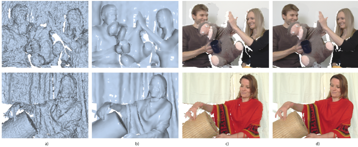
Figure 9: Additional representative results of geometry fusion and texturing from a multi-hybrid camera setup. Raw geometry (a) and its textured version (c). Refined geometry (b) and its optimized textured version (d) obtained by our approach.
