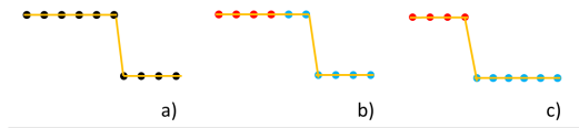
Figure 5: Conceptual approach of our boundary refinement on a 1D example. The dots represent the data points and the MLS resulting curve is shown in orange. a) Depth discontinuity. b) The color information of the data points (obtained from the color image) reveals that the discontinuity is inaccurate. c) Our method robustly classifies the points around the depth discontinuity as local foreground/background.
