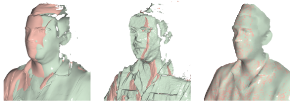
Figure 11: Data from each depth sensor processed individually and then combined, resulting in an inconsistent surface. Richardt et al. [RSD*12] (left). Lang et al. [LWA*12] (middle). Our result: MLS-based reconstruction jointly fusing the geometry from all depth sensors (right).
