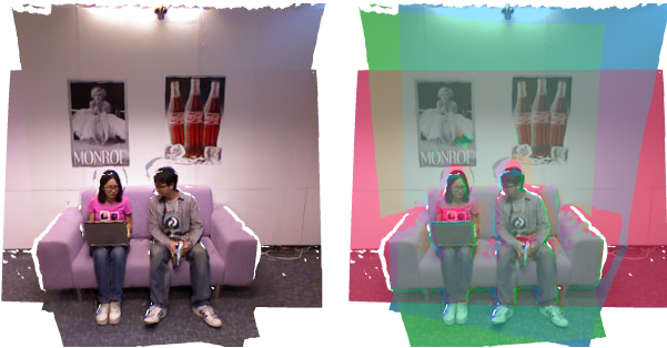
Fig. 8. Left: Representative result with three Kinects. Right: color coded visualization of the overlap of the three Kinects.
