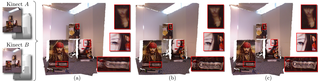
Fig. 2. Registration of two textured geometries acquired from two RGBD cameras (Kinects) by a single 3D rigid transformation (e.g., obtained by the popular ICP algorithm) with (a) the internal parameters of the RGBD cameras provided by the manufacturer, and with (b) the internal parameters computed by Herrera’s calibration toolbox [6]. (c) The proposed 3D registration field with the internal parameters provided by the manufacturer. This comparison shows that, in contrast to single 3D rigid transformation-based methods, our proposed approach provides a visually appealing alignment even when using low accuracy internal (e.g., manufacturer’s) parameters.
