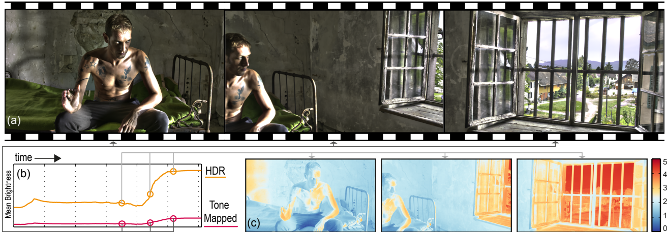
Figure 1: Our method allows local tone mapping of HDR video where the scene illumination varies greatly over time, in this case more than 4 \log_{10} units (c). Note that our method is temporally stable despite the complex motion of both the camera and the actor (b), and the resulting tone mapped video shows strong local contrast (a). The plots show the logmean luminance of the HDR video and the mean pixel values of the tone mapped video.
