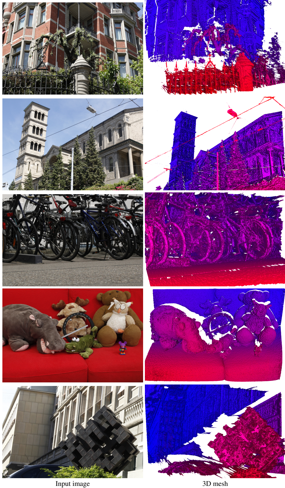
Figure 4: Visualization of 3D meshes (color coded: red near, blue far). From top to bottom: Mansion, Church, Bikes, Couch, and Statue.
