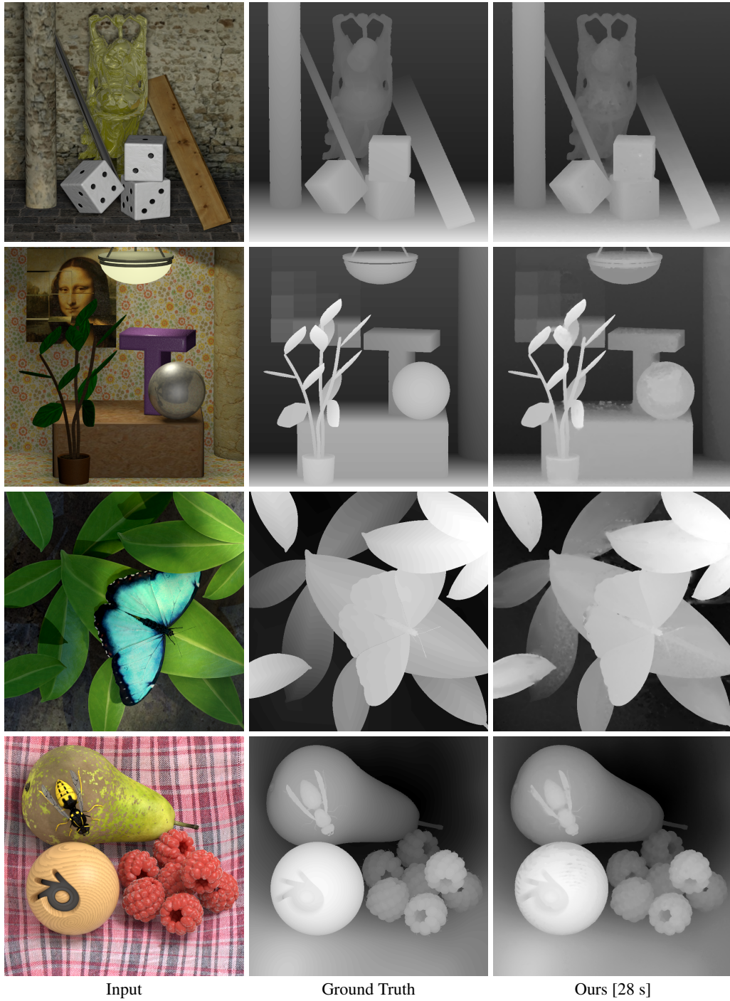
Figure 3: Results on 4D HCI light field data with ground truth. From top to bottom: Buddha, Mona, Papillon and StillLife.
