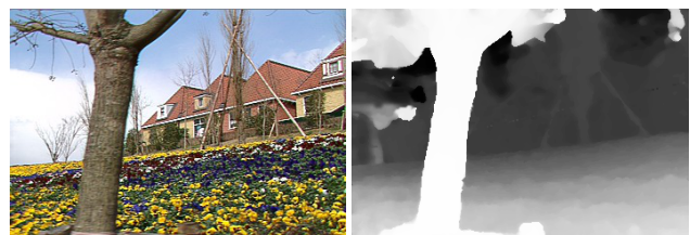
Figure 11: Result on the flower garden sequence with 50 images. Left: One input image with 0.08 MP resolution. Right: Our depth map. The computation time was 3 seconds.
