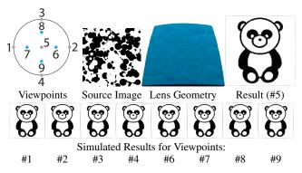
**Figure 14:** We induce a stable viewing zone by exploiting multiview lens generation in a novel way: by using the **same** target images at each of the nine views, arranged in the layout on the left. The lens consists of  $128 \times 128$  facets.
