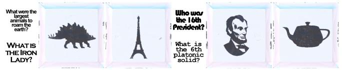
Figure 16: A single source-optimized lens (128×128 facets) encodes four hidden pictographic answers to four textual questions (simulated).
