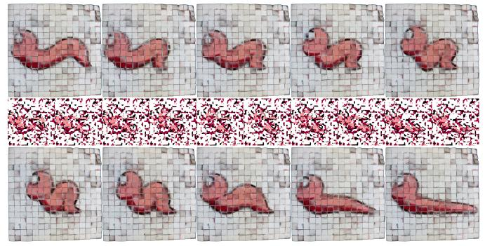
**Figure 9:** Warping an unstructured video sequence with a universal lens with  $16 \times 16$  facets. The middle row has the different (shrunken) source images, and the top and bottom rows are photographs of a manufactured lens placed over the source images as they animate.
