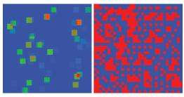
**Figure 7:** Heatmap for a source-optimized lens (left) with values from 0 (blue) to 18 (red) overlaps. Clearly, several facets are matched to the same source patch. The heatmap for a universal lens (right) illustrates the injective mapping: red corresponds to a single match and blue to no match.
