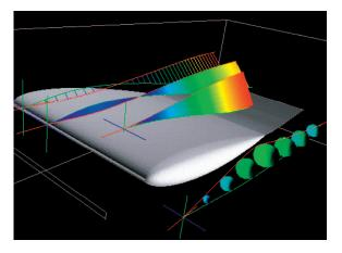
**Figure 3:** Comparing streamlines of two datasets simulated using different turbulence models. The streamlines are compared using line glyphs, strip envelopes, and sphere glyphs to highlight the differences between them. Image Courtesy of Alex Pang [VP04].
