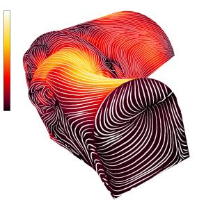
**Figure 2:** Evenly-spaced streamlines on the surface of a gas engine simulation. Perspective foreshortening is utilized and the density of streamlines further away from the viewpoint is increased [SLCZ09].
