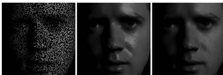
Figure 1 (Left) A set of surface splats; (Middle) point-based rendering with bidirectional reflectance distribution function; (Right) point-based rendering with bidirectional surface scattering reflectance distribution function.
