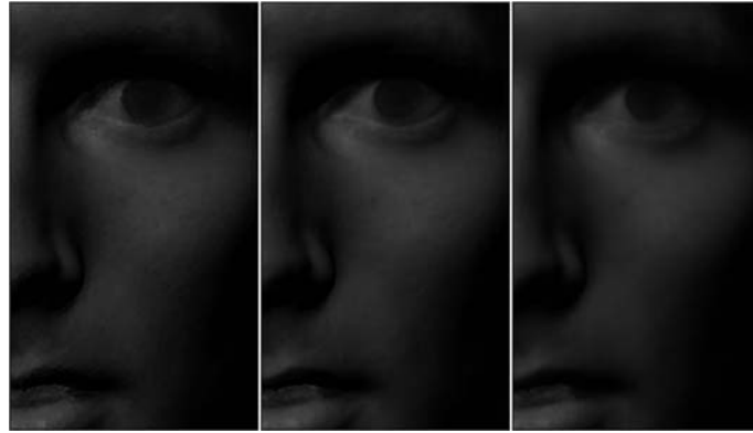
Figure 7 (Left) Elliptical-shaped points rendering; (Middle) high-quality surface splatting; (Right) our results: high-quality surface splatting incorporating subsurface scattering effects.
