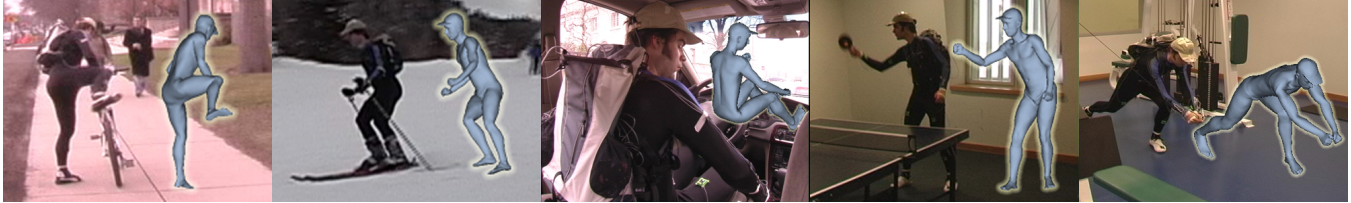
Figure 1: Traditional motion-capture systems excel at recording motions within lab-like environments but struggle with recording outdoor activities such as skiing, biking, and driving. This limitation led us to design a wearable motion-capture system that records human activity in both indoor and outdoor environments.
