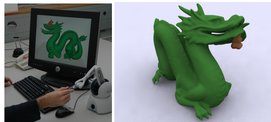
Figure 1: Interactive Deformation with Self-Collisions. A dragon with 13480 triangles deforms interactively (almost 10 fps on average), with accurate handling of self-collisions.
