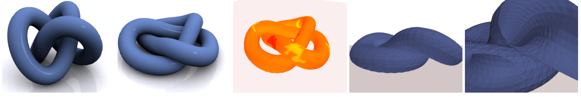
Figure 5: Self-Collisions in a Knot. A knot with 42254 triangles and a 7-mesh hierarchy (119399 tets in M_1 ) is dropped and suffers large self collisions. The middle image shows the resolution near the surface (‘yellow’ is coarse, ‘red’ is fine), achieving smooth deformations and accurate handling of contact boundary conditions. Table 2 evaluates collision detection performance.
