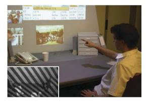
Fig. 12. Projected display containing imperceptible pattern (see inset).
