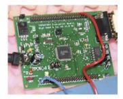
Fig. 4. Microcontroller for generating clock signal.
