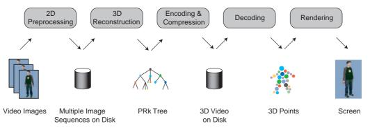
Figure 1: System Architecture of the 3D Video Recorder. The pipeline illustrates the process for one frame.
