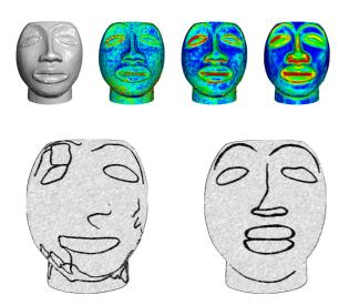
**Figure 12:** Multi-scale feature extraction (bottom right) is superior to single scale extraction (bottom left) on a noisy range scan. The top row shows the original point cloud and variation estimates for different scales.
